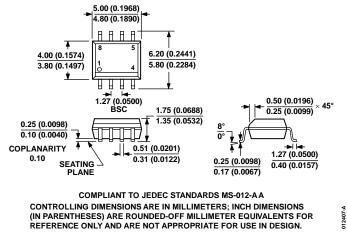
ERENCE ONLY AND ARE NOT APPROPRIATE FOR USE IN DESIGN. Figure 40. 8-Lead Standard Small Outline Package [SOIC\_N] Narrow Body (R-8)
