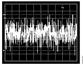
Figure 10. Input Voltage Noise (20 nV/Div)
