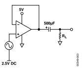
Figure 3. Test Circuit for Figure 4, Figure 5, and Figure 6
