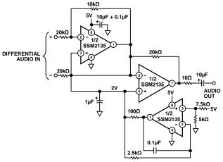
Figure 36. Single-Supply Balanced Differential Line Receiver
