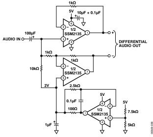
Figure 35. Single-Supply Differential Line Driver
