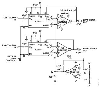
Figure 39. Single-Supply Logarithmic Volume Control
